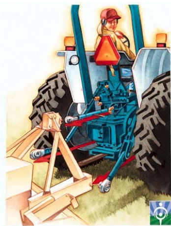
Figure 5.3.a. Back slowly to the implement to be attached. Using the hydraulic controls, raise or lower the draft arms to nearly match the implement's lower hitch pins.
