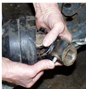
Figure 5.3.e. A firm grip will be needed to press in on the detent lock of the PTO shaft. This lock engages the groove in the stub shaft to secure the PTO driveline shaft to the stub shaft. Other forms of locking the PTO shaft will be found in Task Sheet 5.4.
